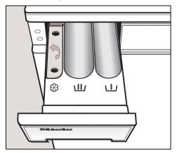
■ Place the recommended amount of detergent into the main wash compartment Ш. If "Heavy Soil" is selected, add ¹/₄ of the total amount of detergent to the Ш compartment. Place fabric softener or liquid starch in compartment %.
